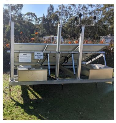
Figure 4 – Delta Coal BarnOwl - Real-time directional noise monitor.
